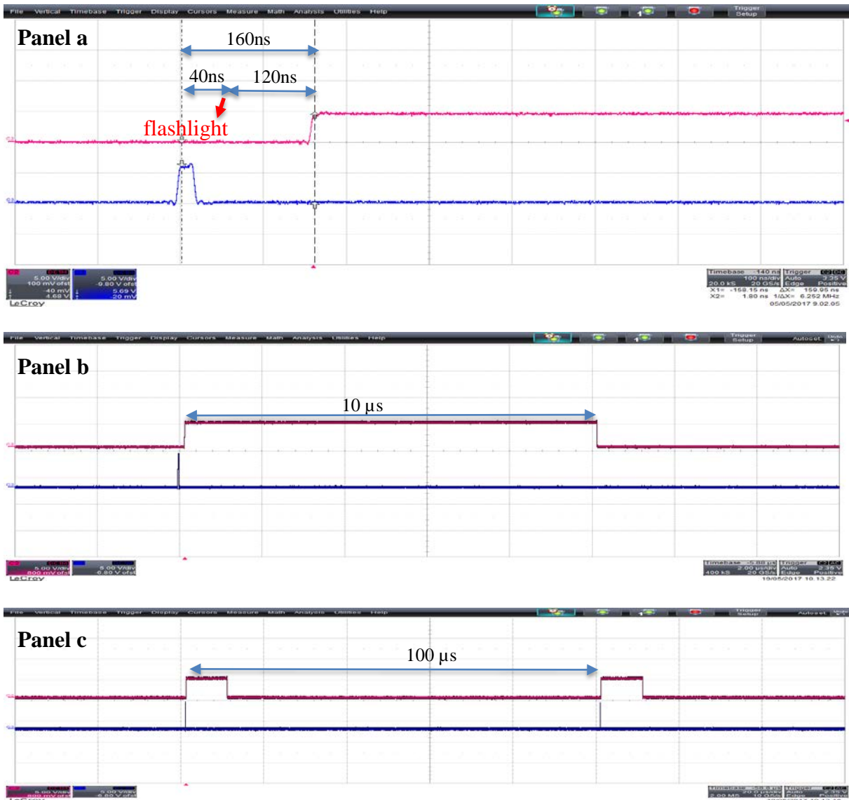
Figure 11. Panel a) HOLD (red waveform) and TRIGGER (blue waveform). To be noted the total 160ns delay respect to the TRIGGER signal. Additional 40ns are required by the pulsed light sources to be ready for firing. Panel b. The duration of the HOLD signal before to go down is 10µs, in fact we select this for the “Read” signal. Panel c) The repetition time is 100µs meaning 10 KHz or 10000 pulses/s.
